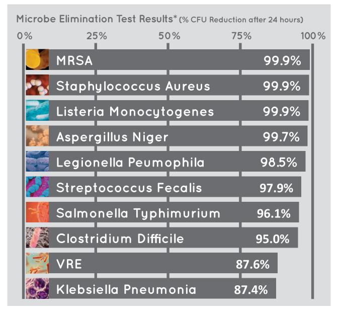
\*In an independent lab test, 10 common microbes were selected, and each of them was incubated on panels for 24hrs at 37°C and >90% RH. As the table shows, AM-Clad panels demonstrate high antimicrobial activity. Use of AM-Clad, along with an adequate cleaning regime, would significantly reduce microbial growth, including dangerous pathogens.
